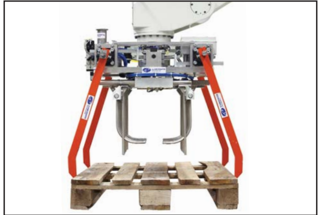
Pallet pick arms in operation
