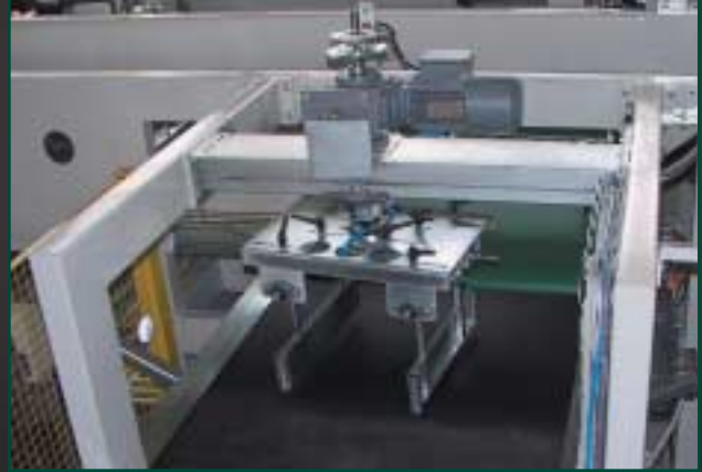
Electromechanical devices turn the incoming bags by 90°
