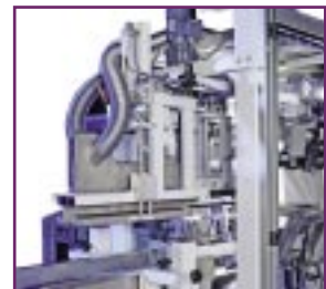
Secondary de-aeration system to press the air out of the bag top.
