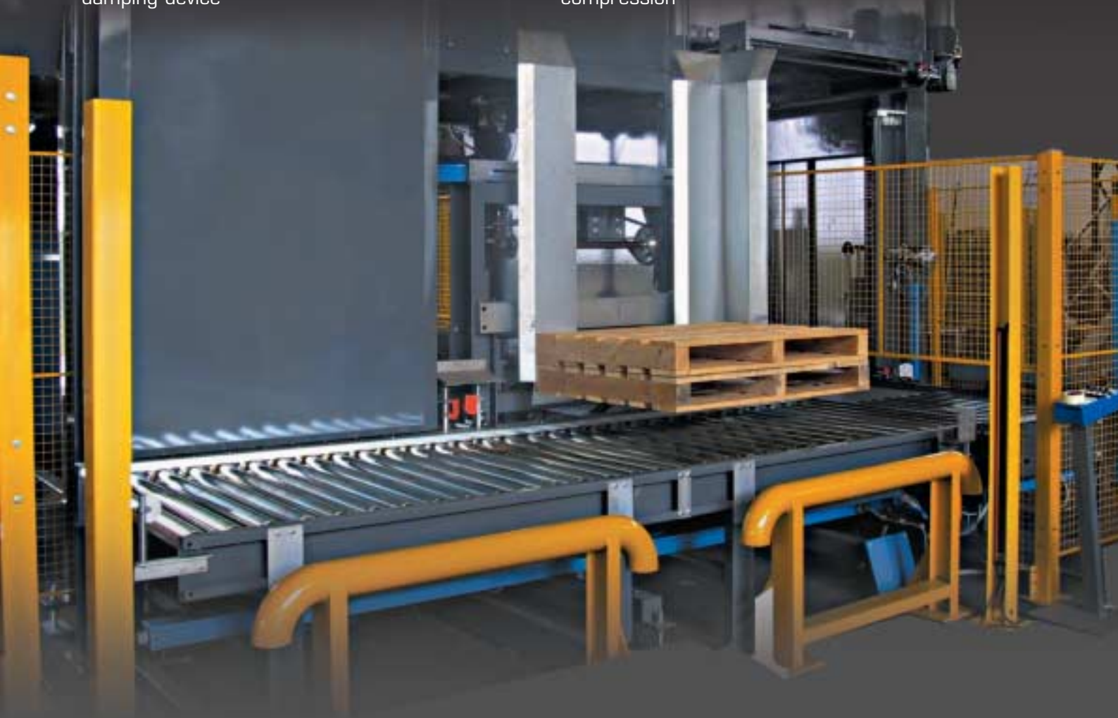
Bag pressing device as bag flattener with damping device
