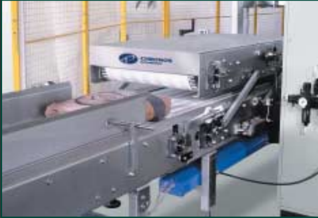
Bag pressing device as bag flattener with damping device
