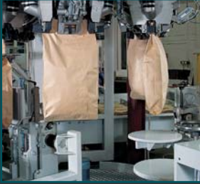
Filling and compacting
